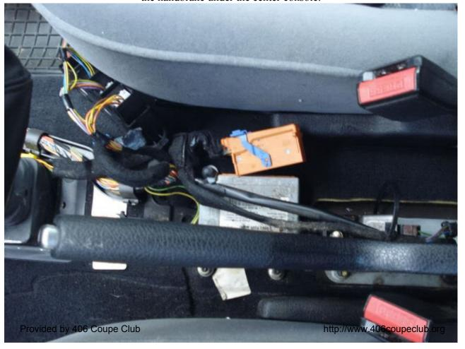
The connector is held in place by that blue lever thing, you have to turn/pull it anti-clockwise and the connector comes out with it. I found that you can undo it without removing the console, to save fiddling about with wires, but it's probably easier if you do.
